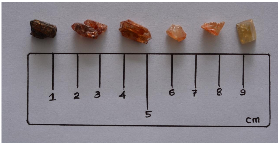
Fig. 5: Reddish brown zircon before heat treatment and range of colours produced after heat treatment
